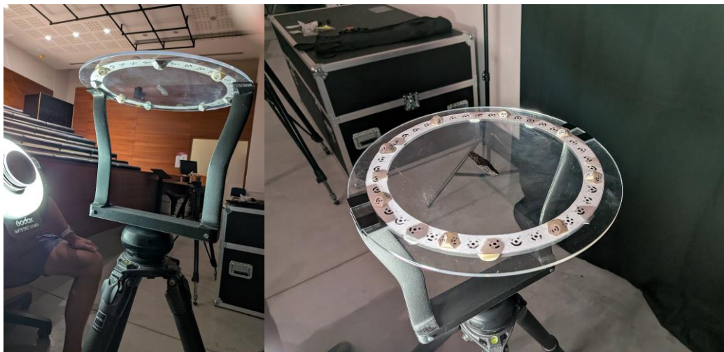
Figure 4 - Circular PMMA support used for the reference acquisitions: bottom view with visual patterns for photogrammetry (left), and upper surface of the Plexiglas support.
