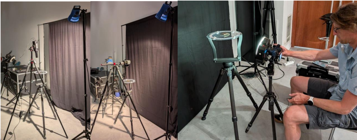
Figure 3 - HSI and photogrammetry set-up. HinaLea VNIR 4250 hyperspectral camera (left), Specim IQ hyperspectral camera (centre) and Nikon Z7 II camera for photogrammetry (right).
