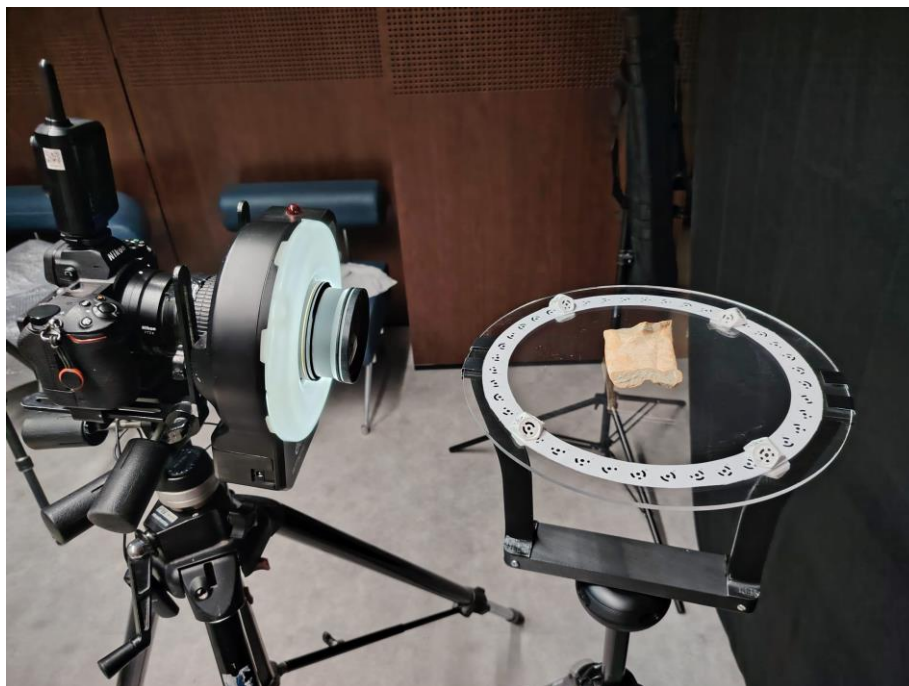
Figure 3.1: Photogrammetry setup with the rotating support and coded targets
