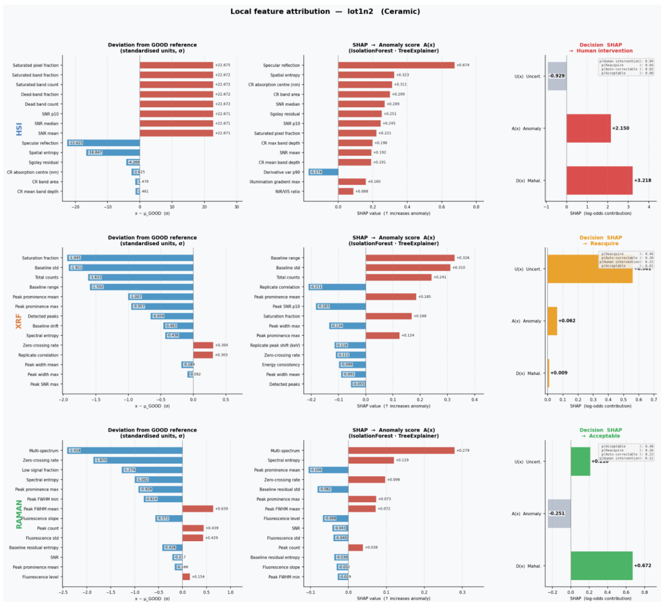
Figure 8.1: Local feature attribution analysis using local XAI methods, illustrating the contribution of individual features to classification outcomes, for one ceramic and one lithic artefact. The plots highlight how different features positively or negatively influence the decision process, revealing the underlying causes of quality degradation and supporting the interpretability of the calibration pipeline.
