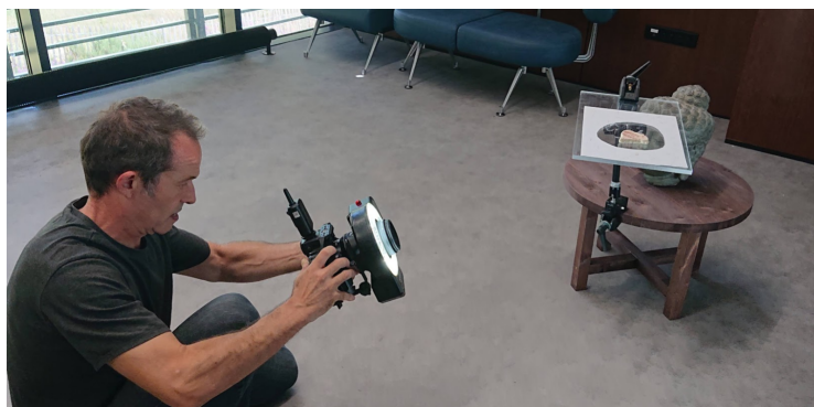
Figure 1 - Taking manual pictures of an object for photogrammetry at Archeovision
