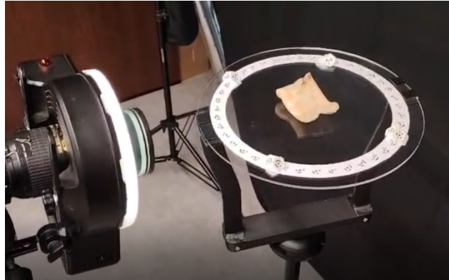
Figure 3 - Last support designed by Archeovision for photogrammetry
