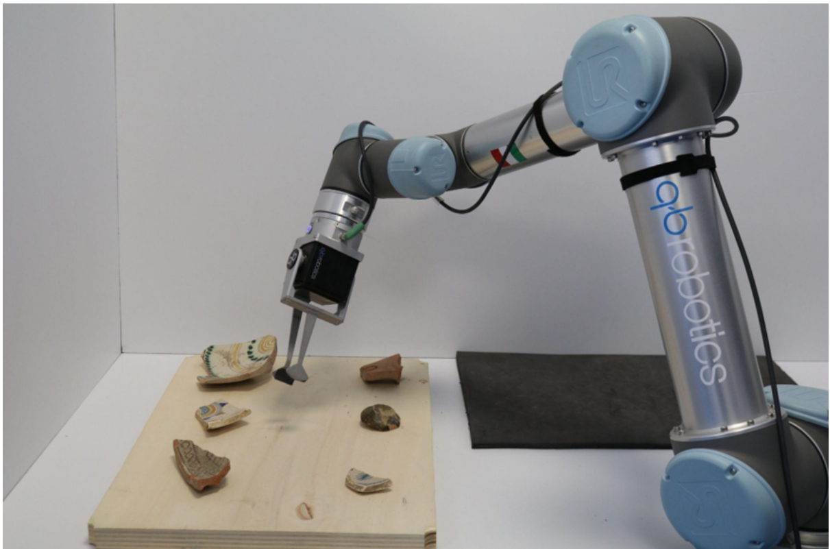
Fig. 8: Experiments with qbSoftClaw and customized fingers.
