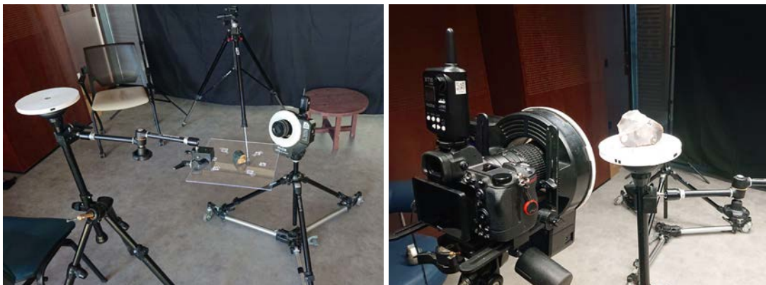
Fig. 6 - Acquisition tests performed with a transparent tray (on the left) and recognition targets or on a solid rotating platform (on the right).
