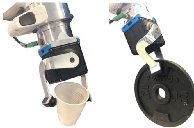
Fig. 9: SoftClaw with deflection control: soft grasp on the left and strong grasp (high deflection reference) on the right side.
