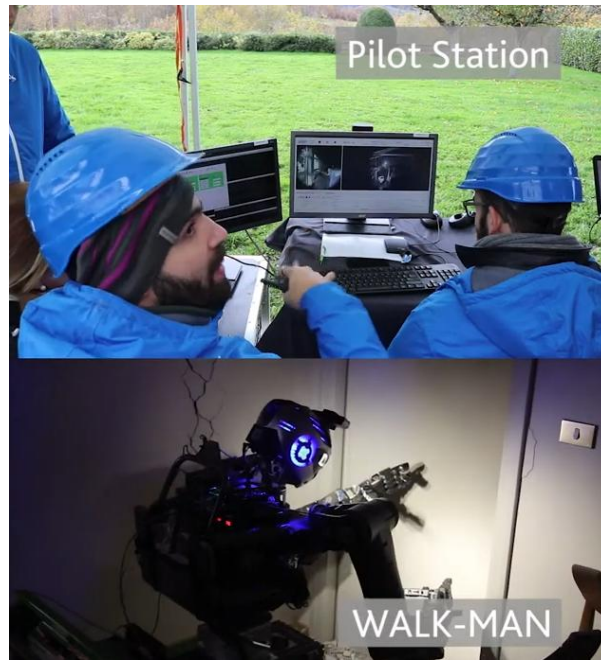
Fig. 4 - Field Experiments in a Post-earthquake Scenario with WALK-MAN, a Humanoid Robot, in Amatrice, Italy. On the top line, the pilot station is visible, while on the bottom line, the robot WALK-MAN executes the commanded actions.
