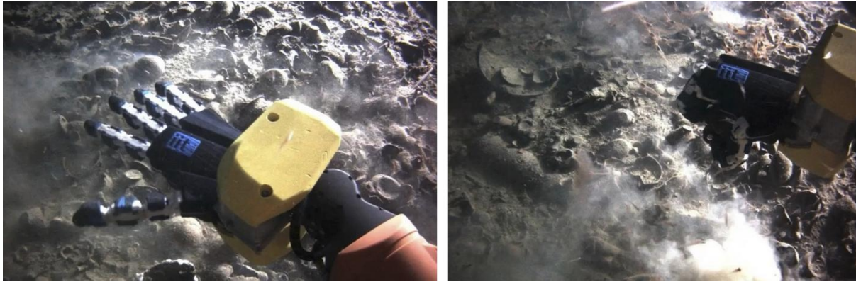
Fig. 2 - OceanOneK: Pisa/IIT SoftHand grasping archaeological artefacts during the 2022 Corsica Expedition.
